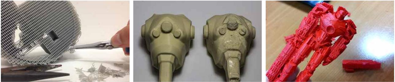
**Fig. 4** Problems in the support removal process
