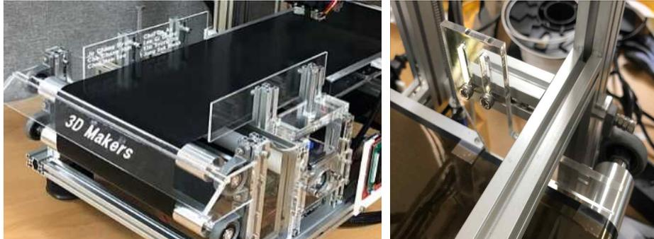
**Fig. 21** Conveyor belt and belt guide
