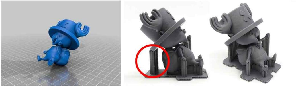
**Fig. 3** The generation of support for objects in the air
