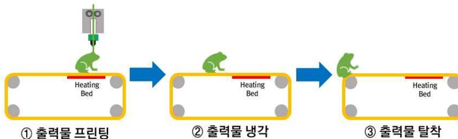
Fig. 37 Schematic diagram of conveyor belt driving system
