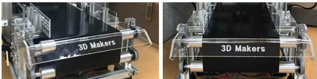
**Fig. 23** Fabrication of support for detaching output
