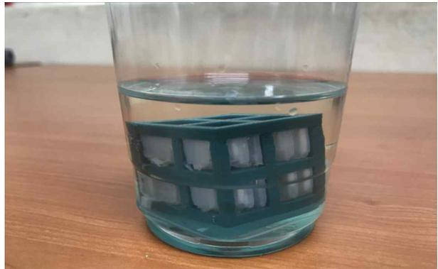
**Fig. 41** Support removing process
