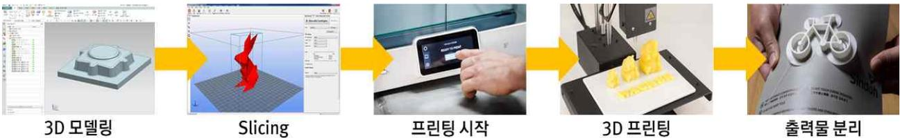
Fig. 2 Process of 3D printing
