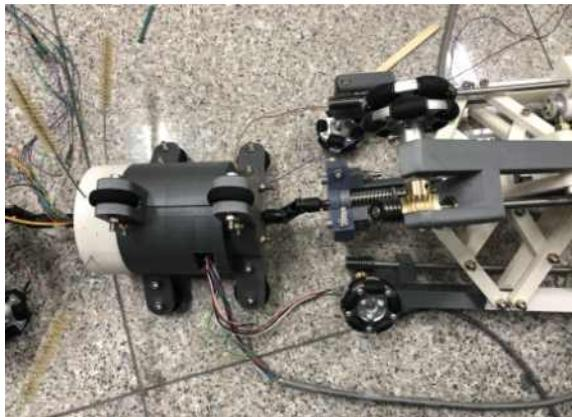
Fig. 109 Fastening the rear drive using the previous mechanism(1)
