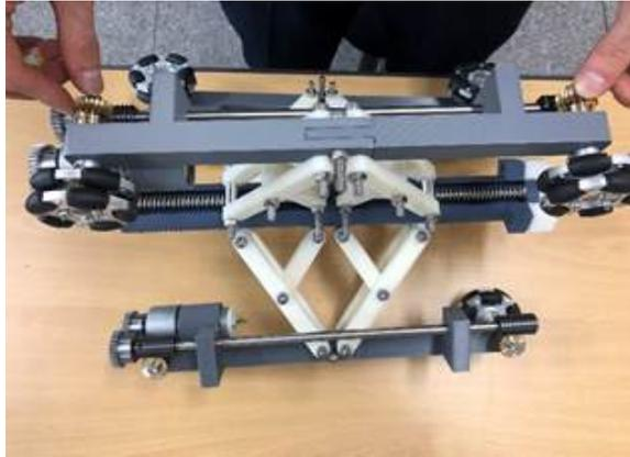
Fig. 93 Single driving part unit(1)
