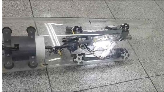
Fig. 118 Straight drive in the pipe
