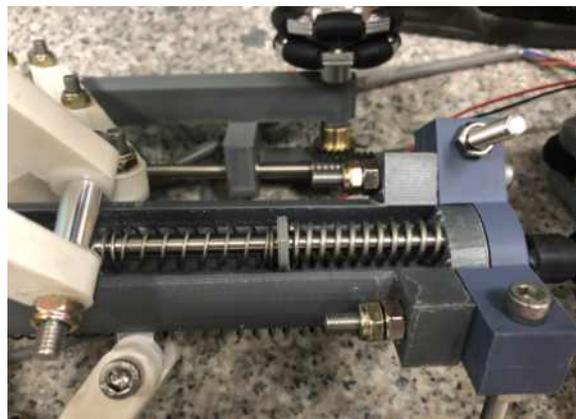
Fig. 92 Two compression springs with different stiffness
