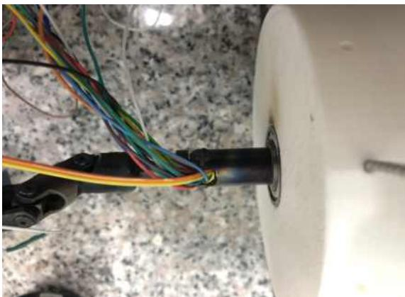
Fig. 103 Insertion of wires in pipes to prevent twisting of wires
