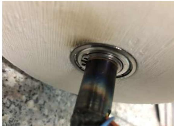
Fig. 102 Bearing and snap ring fastening
