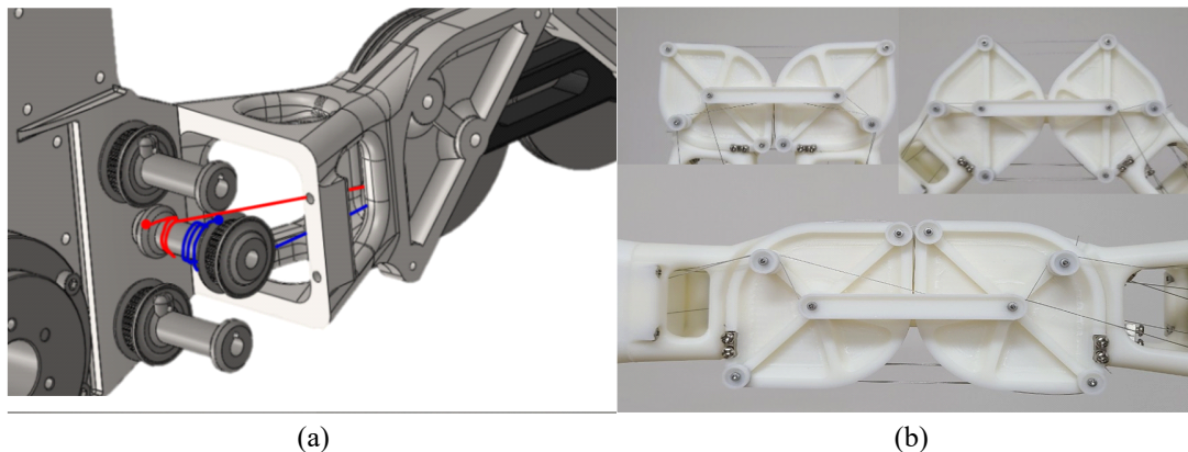
Fig. 2 Detailed design of elbow joint: (a) wire pulley and wire connection for elbow part; (b) elbow design with wire mechanism
