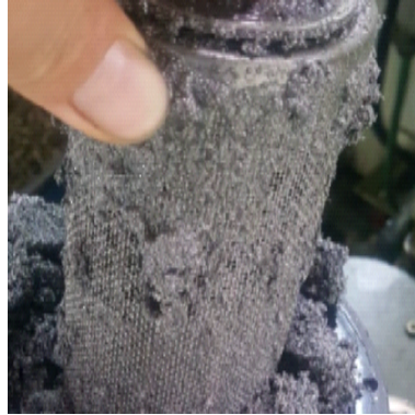
Fig. 1 Contamination of mesh filter mounted on pump (2)
