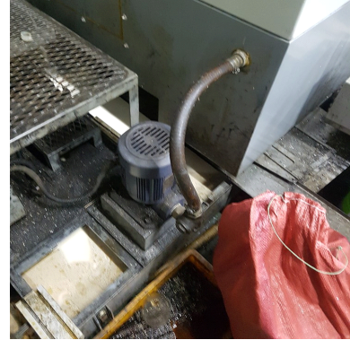
Fig. 2 Broken cutting oil pump
