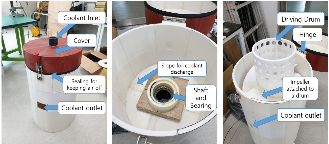
Fig. 15 Completed body using 3D printer
