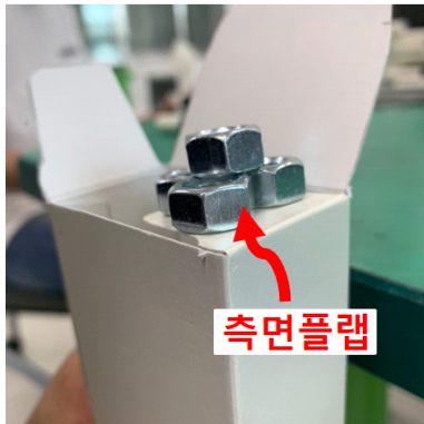
Fig. 30 Nuts required for side flap ground 5EA
