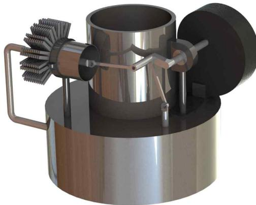
Fig.10 Ducts including Stirling Engine
