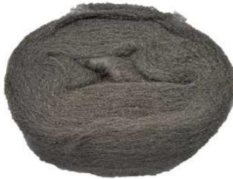
Fig.9 Regenerator(Steel Wool)
