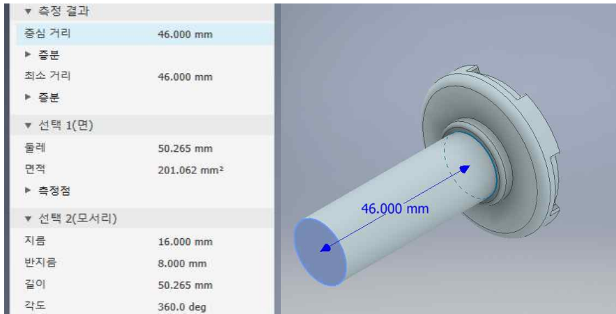
Fig. 19 Dimension of main shaft made of SUS-304 Stainless Steel
