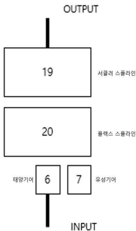
Fig. 15 gear reduction ratio
