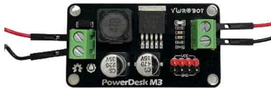
Fig. 18 DC/DC converter
