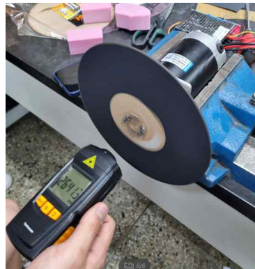
Fig 20 Measurement of Disc RPM
