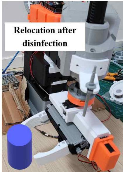
Fig. 21 Robot gripper motion (Using servo motors)
