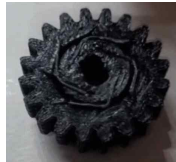
(b) Gear with actually manufactured anti-reversal device
