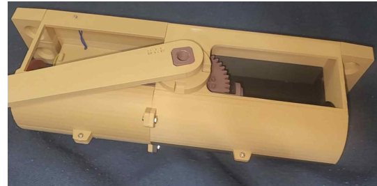
(b) External shape of prototype of improved door closer
