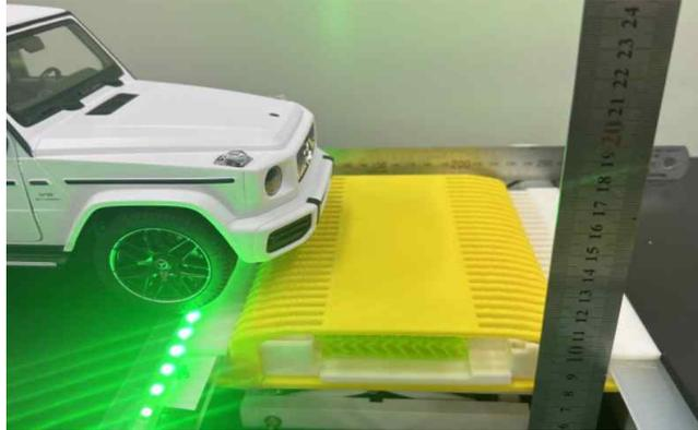
Fig. 24 The green LED light bar attached on the speed bump
