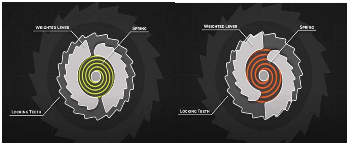
Fig. 8 Principle of Seat Belt Locking
