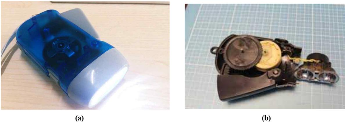
Fig. 22 (a) The picture of self-powered flashlight (b) The internal structure
