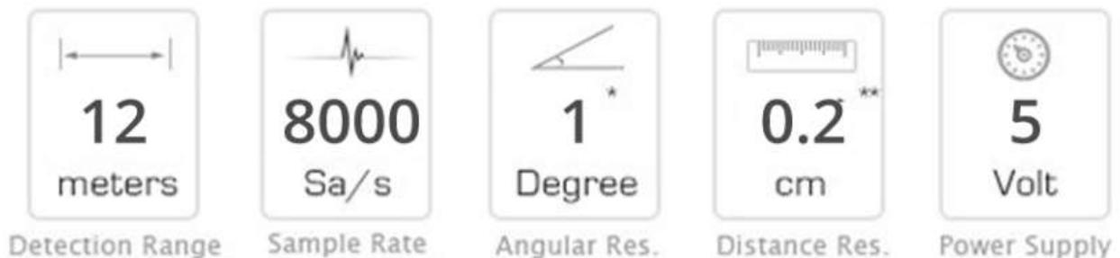
Fig. 7 RP Lidar-A1 specifications
