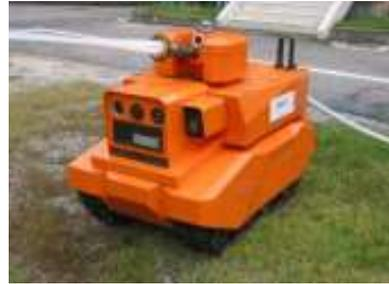
(b) Firefighting robot using caterpillar
