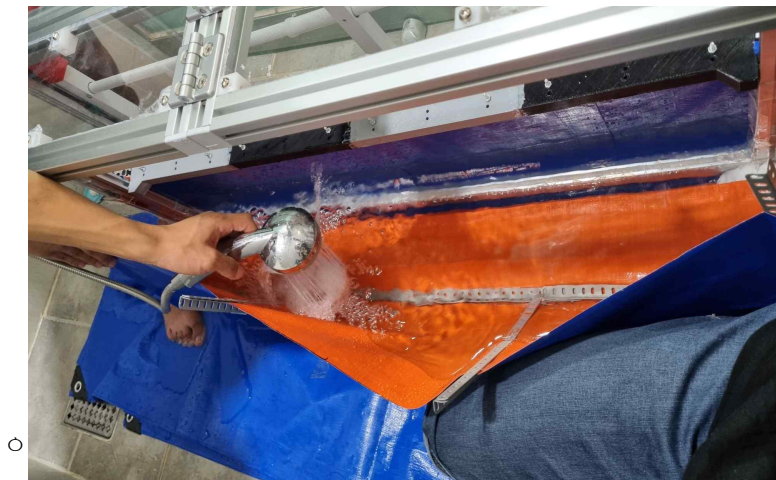
Fig. 8 Water barrier test
