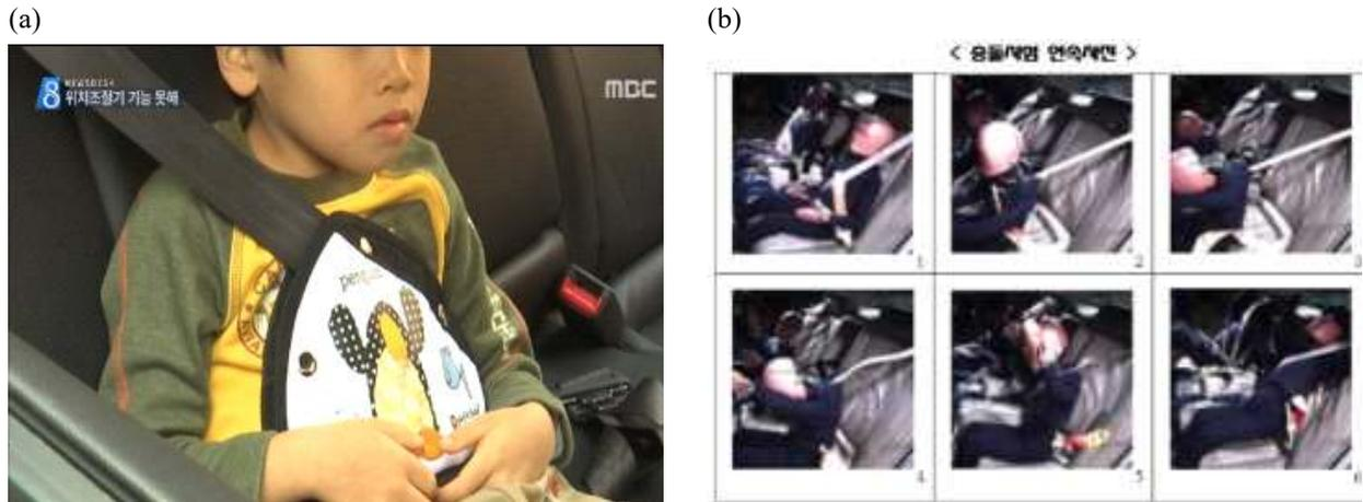
**Fig. 2** (a) Child Seatbelt Positioning Regulator and (b) Collision test continuous picture
