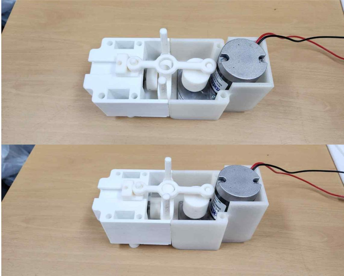
Fig. 29 Appearance of the device when the bike is locked
