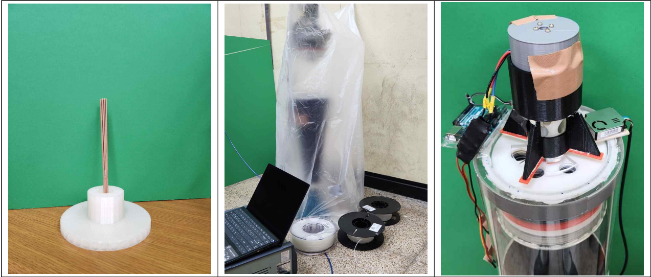
Fig. 9 Particulate Matter Generation through incense burning (left), Air Purification Validation Test Set-up (Middle), PM Sensor Installed at the outlet (Right)
