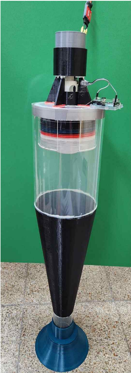
Fig. 12 Cyclone dust collector empowered by Tesla compressor
